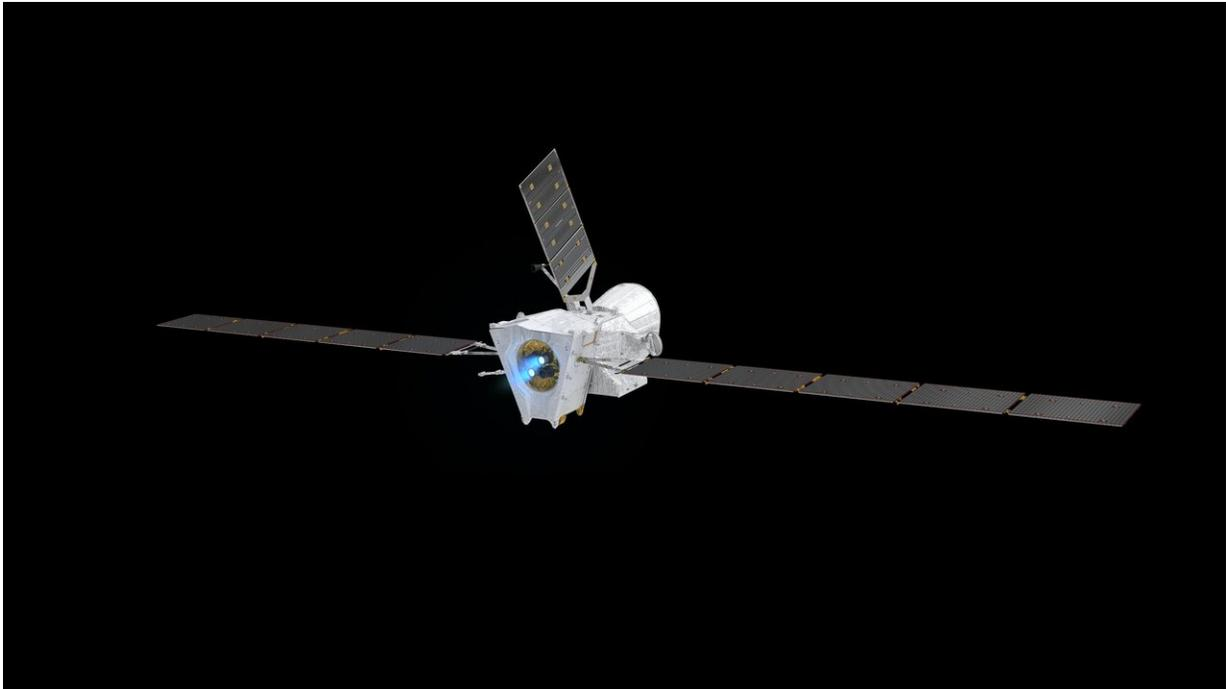
The Mercury Transfer Module (foreground, with two large solar wings) carries the Mercury Planetary Orbiter (middle, with one solar wing pointing up) and the Mercury Magnetospheric Orbiter (hidden inside the solar shield, on the far side) to Mercury. Credit: ESA/ATG medialab
