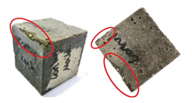
A compound, called CAOXY, that forms when road salt interacts with concrete is behind the deterioration of road surfaces and the formation of potholes. Drexel University researchers are trying to thwart CAOXY formation using a special kind of bacteria. Credit: Drexel University
