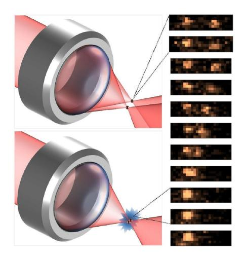
As the two lasers move together, the atoms interact with each other and exchange properties. Credit: University of Otago
