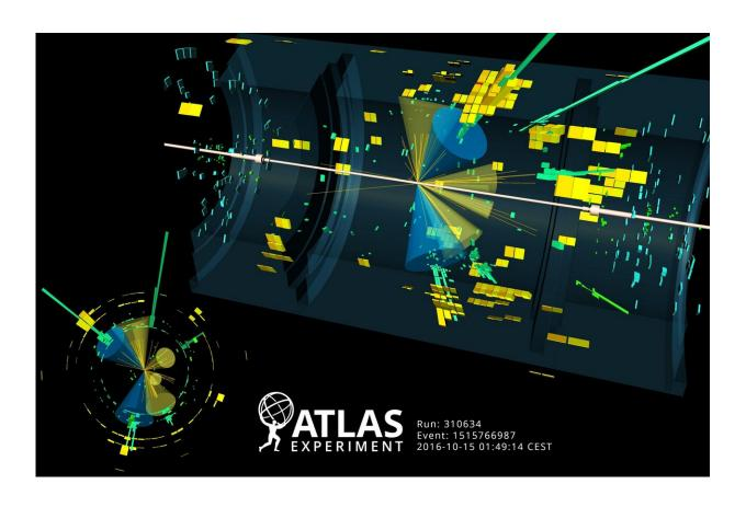
Visualisation of an event from the  $t\bar{t}H(\gamma\gamma)$  analysis. The event contains two photon candidates (green towers), while the b-jets are shown as yellow (blue) cones. Credit: ATLAS Collaboration/CERN
