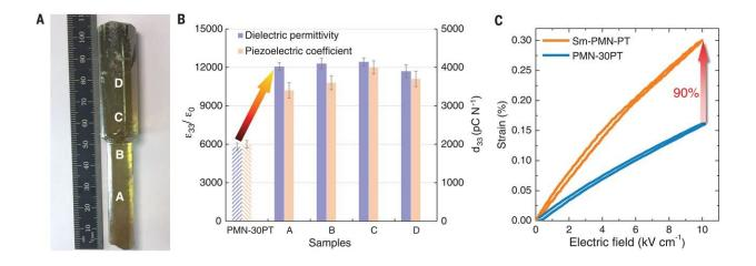
Image and electromechanical properties of [001]-oriented Sm-doped PMN-PT crystals. (A) Image of as-grown Sm-PMN-PT crystal. The compositions of points A, B, C, and D are listed in table S1. (B) Dielectric and piezoelectric coefficients of Sm-PMN-PT crystals versus those of PMN-30PT (patterned). (C) Electric field—induced strains for Sm-PMN-PT (sample B: 0.66 mol % Sm-doped PMN-30PT) and PMN-30PT crystals. Credit: *Science* (2019). 10.1126/science.aaw2781
