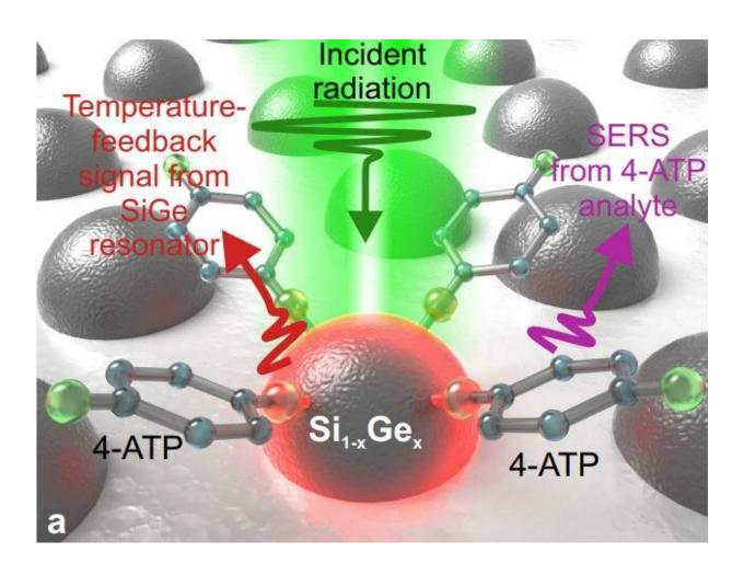
Artistic representation of the alloyed Si1?xGexnanoparticles with 4-ATP molecules adsorbed on their surface. IsolatedMie nanoresonator is pumped with laser radiation resulting in SERSfrom the attached molecules as well as Stokes Raman yield related toSi1?xGex lattice phonons, which provides information on
