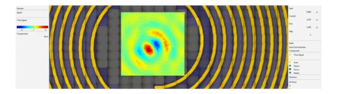
Movie showing an animation of the vortex measured experimentally with a laser interferometer. Colors correspond to the amplitude of the normal displacement at the surface of the coverslip. Credit: Science Advances, doi: 10.1126/sciadv.aav1967
