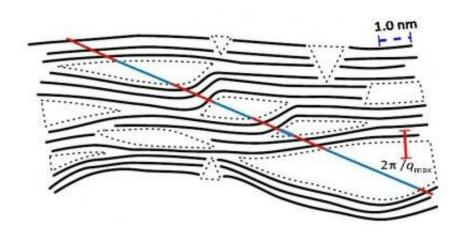
Schematic view of carbon structures with pores. Credit: HZB
