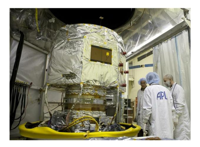
In late 2010, engineers at the Johns Hopkins Applied Physics Laboratory prepare to place Van Allen Probes spacecraft "B" in a thermal-vacuum chamber, where the propulsion system would be tested to ensure it could stand up to the range of
