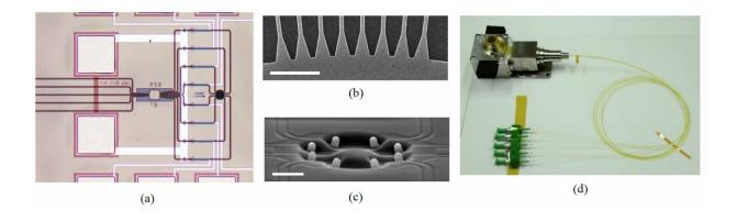
The multiplexing/demultiplexing module fabricated (a,d) employs a property of light called the "optical vortex" to transmit/receive multiple signals simultaneously through a shared optical medium. The required light waves with different optical vortexes are generated using a combination of a star coupler (b) and an optical-vortex generator (c). Credit: The Optical Networking and Communication Conference & Exhibition 2019
