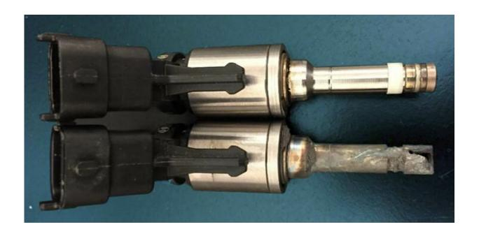
A fuel injector can be heavily damaged by a pre-ignition event (bottom); a new injector is shown above. Credit: Eshan Singh
