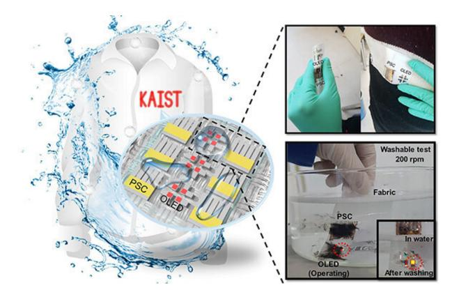
Figure 1. Schematic and photo of a washable wearing display module. Credit: The Korea Advanced Institute of Science and Technology (KAIST)
