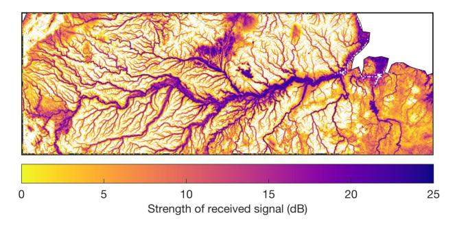
In the second phase, the CYGNSS mission has expanded to include land-based studies. In the prime mission, a surprising capability emerged -- CYGNSS can characterize flooded landscapes and measure subsurface soil moisture, as seen in this CYGNSS map of the Amazon basin. Credit: University Corporation for Atmospheric Research/University of Michigan
