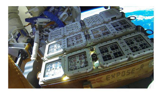
The EXPOSE-R2 experiment system with BIOMEX on the ISS. Credit: German Aerospace Center
