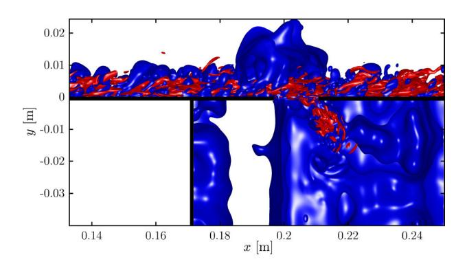
At the top, vorticity isosurfaces ( $\pm$  3,000 Hz, colored blue and red) of the turbulent flat-plate flow are visible. Below the flat-plate flow, the rectangular box of the resonator is mounted. Credit: Lewin Stein, TU Berlin.
