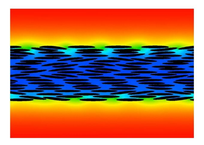
Visualization of CMC densification depicting poor infiltration (blue) with internal voids. Credit: Ramanan Sankaran
