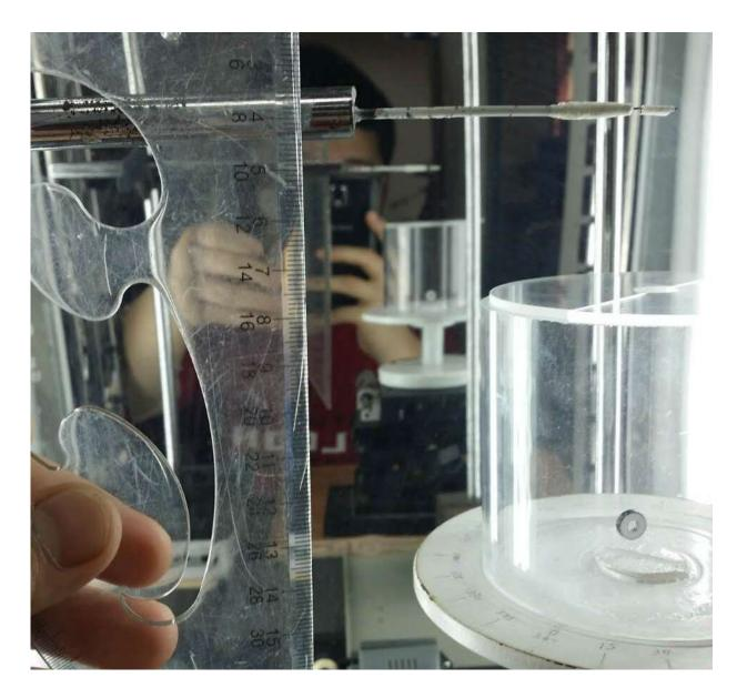
Torsion pendulum made of spider dragline silk. Credit: Liu et al., Sci. Adv. 2019; 5 : eaau9183
