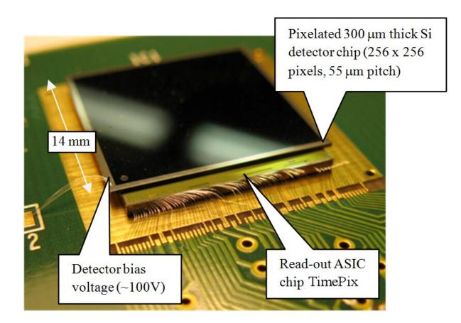
The Timepix chip sensor was originally developed through CERN's Medipix
