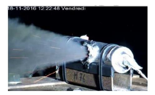
To simulate a micrometeoroid impact an 8 mm bullet was fired into a space battery cell to simulate a micrometeroid impact. Credit: ESA/Airbus
