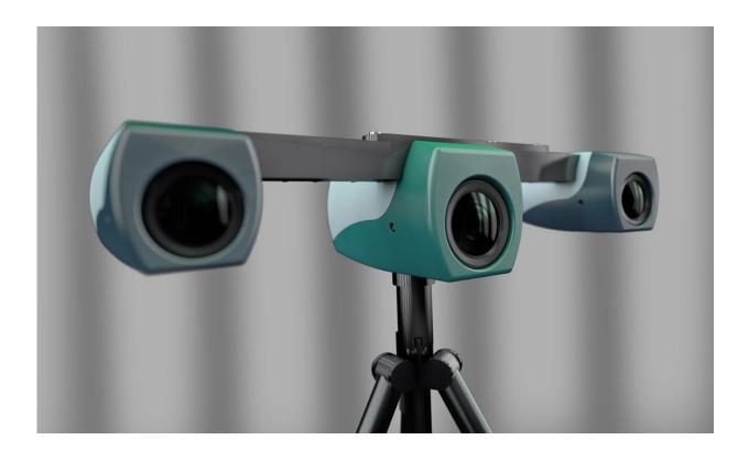
3D sensor technology: two high-speed cameras and a gobo projector capture the 3D data of the moving person. Credit: Fraunhofer IOF
