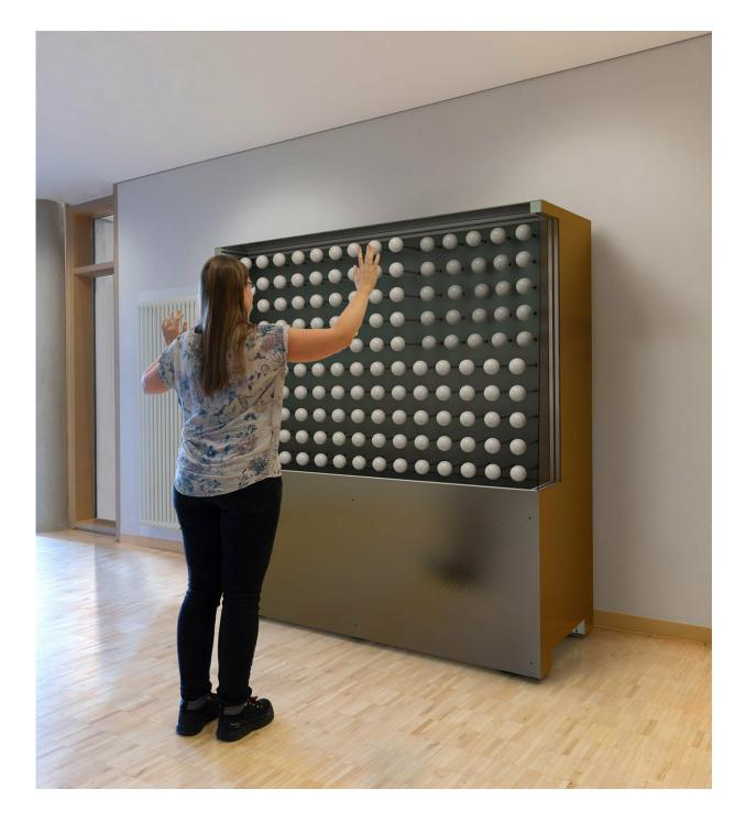
The spheres respond instantaneously to the movements of the person standing in front of the wall. Credit: Fraunhofer IOF
