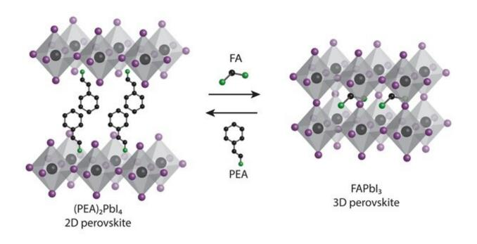
The 2D films based on 2-phenylethylammonium lead iodide produce 3D formamidinium lead iodide films via cation exchange. Credit: Loi lab / University of Groningen
