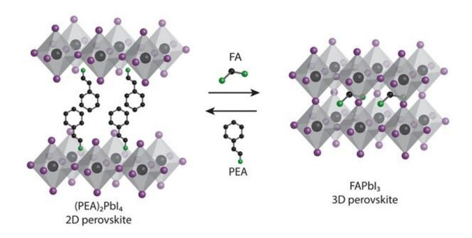
The 2D films based on 2-phenylethylammonium lead iodide produce 3D formamidinium lead iodide films via cation exchange. Credit: Loi lab / University of Groningen
