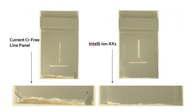
Test results demonstrating areas of 1mm (Intelli-ion) vs. 10mm (control) creep in samples. Credit: Hexigone Ltd
