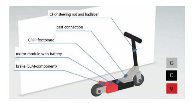
Smart use of materials. G= Casting; C= Composite; V= Processing Technology. Credit: Fraunhofer IGCV
