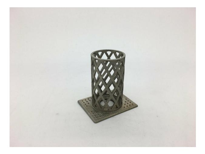
Connecting piece prior to lamination, showing the novel pin structure that helps create a positive bond with the CFRP prepreg. Credit: Fraunhofer IGCV
