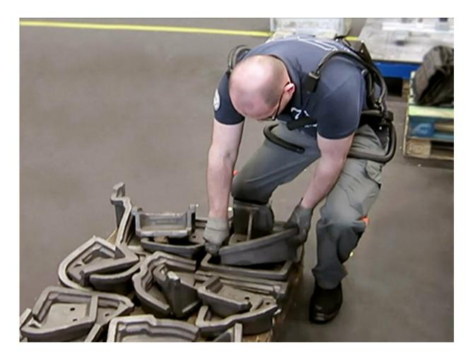
ErgoJack with a locking hip joint and leg brace supports the worker when lifting heavy loads. Credit: Fraunhofer IPK
