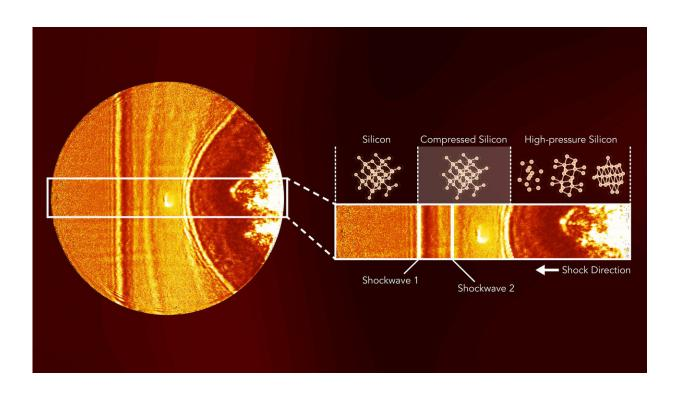
After blasting silicon with intense laser pulses at SLAC's Linac Coherent Light Source, researchers saw an unexpected shock wave appear in the material before its structure was irreversibly changed. Credit: Gregory Stewart/SLAC National Accelerator Laboratory
