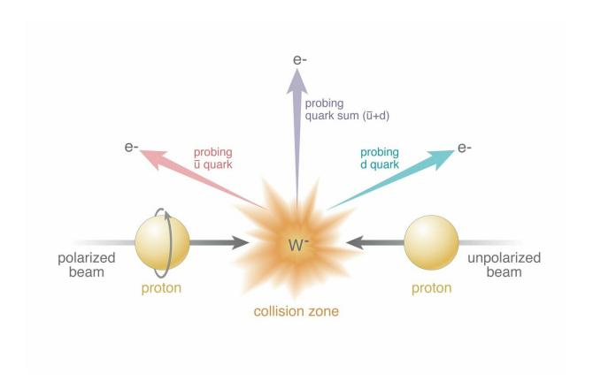
Collisions of polarized protons (beam entering from left) and unpolarized protons (right) result in the production of W bosons (in this case, W-). RHIC's
