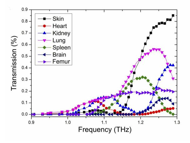
THz medical examination of sections of mice organ tissues for skin, heart, kidney, lung, spleen, brain, and femur. Transmission spectra were measured by rotating the SBE. The spectra revealed different transmission peaks characteristic of the organ tissues. Credit: *Scientific Reports*
