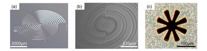
(a) A photograph of the spiral bull's eye (SBE) structure, (b) a microscope image of the double-corrugated devices, and (c) a scanning electron microscope image of the eight-tip Siemens-star aperture at the center of the SBE structure. Credit: *Scientific Reports*
