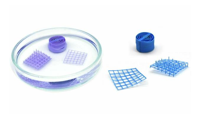
In the dry state (left; here in an anhydrous liquid) the sensor material is purple, in the wet state (e.g. from air humidity) it turns blue. The printed workpieces shown here are each about one centimetre wide. Credit: UAM, Verónica García Vegas
