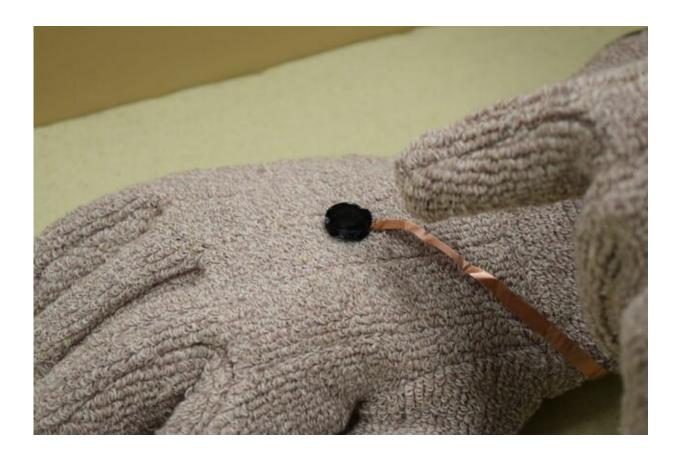
The triboelectric nanogenerator can detect when wearers are in danger or disabled because it can sense the difference between walking, running, jumping and stillness. Credit: UCLA and McMaster University
