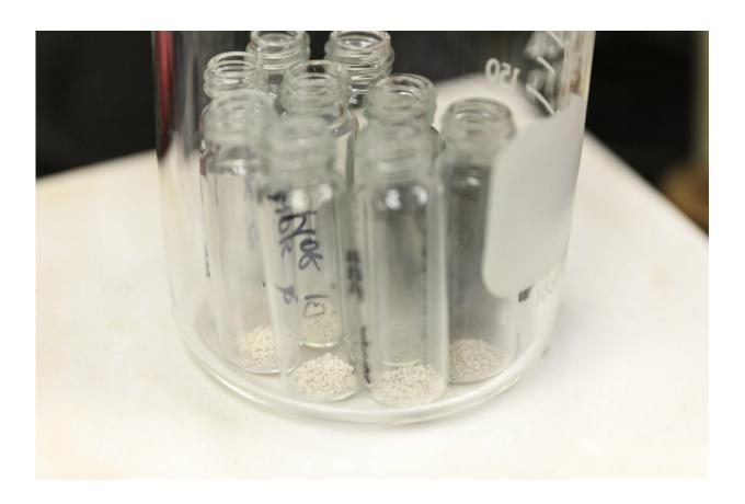
Sand and clay water filter samples were analyzed using neutron scattering and the SNS user laboratories to see how they interacted with water containing the chemical bisphenol A, also known as BPA. Credit: ORNL/Genevieve Martin
