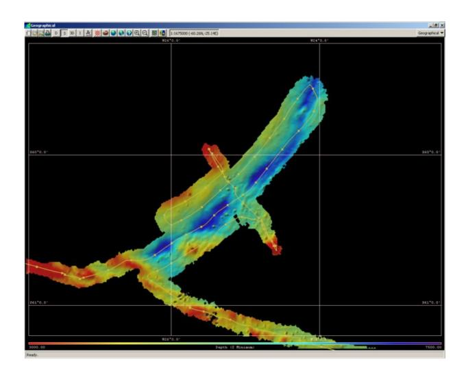
This shows preliminary data from the multibeam (swath) sonar system that maps the seabed beneath and up to 10 km to the side of RRS James Clark Ross. Colour is depth in m (scale at the bottom), and the yellow line is the ship's track. Credit: British Antarctic Survey
