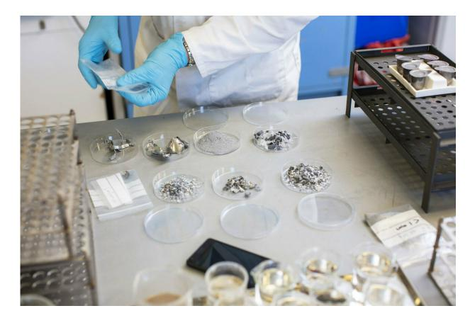
The resulting material is then separated before being mixed at almost 500°C with a powerful oxidizer. They were then able to do a detailed analysis of the resulting solution in acid to determine its precise chemical contents Credit: University of Plymouth
