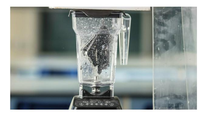
Scientists used a blender to grind a smartphone to dust in order to reveal its precise contents. Credit: University of Plymouth
