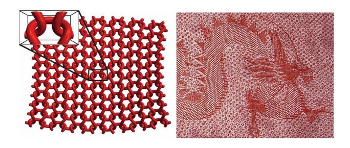
a) Knitting is a periodic structure of slip knots. b) Textiles with intricate patterns are knit by combining slipknots in specific combinations. Credit: Elisabetta Matsumoto
