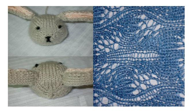
Topological defects in the square can shape the (a) out-of-plane and (b) in-plane deformations of knitted textiles. Credit: Elisabetta Matsumoto
