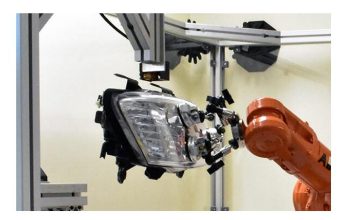
By using a robotic arm to precisely manipulate the headlight under a stationary 3D print head, complex geometries can be printed without the need for support material. Credit: Swinburne University of Technology
