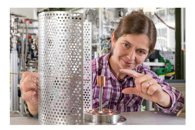
Dr. Eve Stenson uses spare parts to demonstrate the structure of the positron trap: in the center is the permanent magnet. The wire on the left represents a probe that can be inserted into the trap. It allows researchers to determine the quantity of injected particles successfully captured inside the magnetic field. Credit: Axel Griesch / IPP
