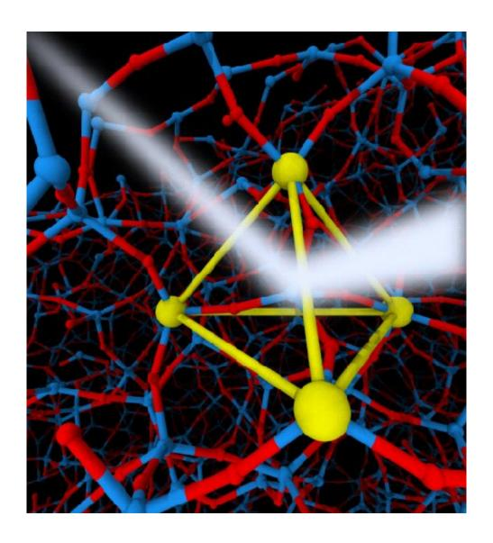
X-ray scattering (white beem) image of local tetrahedral ordering formed by Si atoms (large yellow particles) in liquid silica (Si atoms are large particles and O atoms are small particles) by simulation. Credit: 2019 Hajime Tanaka, Institute of Industrial Science, The University of Tokyo
