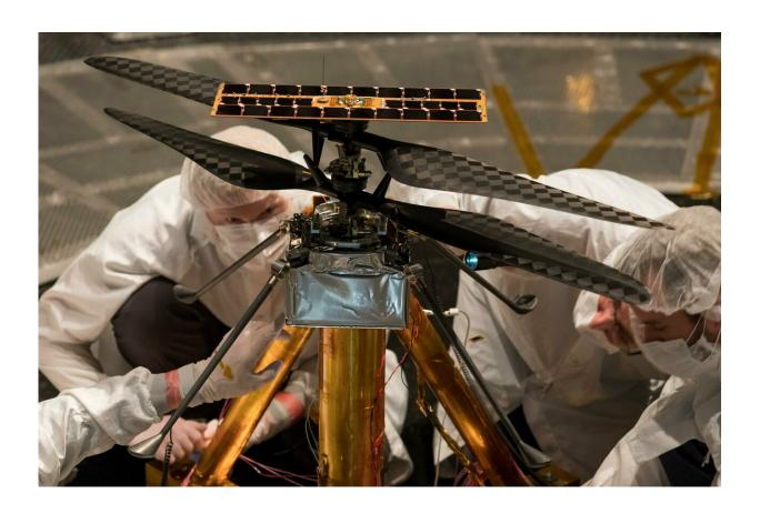
Members of the NASA Mars Helicopter team inspect the flight model (the actual vehicle going to the Red Planet), inside the Space Simulator, a 25-footwide (7.62-meter-wide) vacuum chamber at NASA's Jet Propulsion Laboratory in Pasadena, California, on Feb. 1, 2019. Credit: NASA/JPL-Caltech
