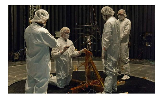
Members of NASA's Mars Helicopter team prepare the flight model (vehicle going to Mars) for a test in the Space Simulator, a 25-foot-wide (7.62-meter-wide) vacuum chamber at NASA's Jet Propulsion Laboratory in Pasadena, California. The image was taken on Jan. 18, 2019. Credit: NASA/JPL-Caltech
