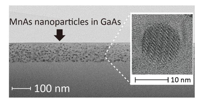
Transmission electron microscope images of MnAs nanoparticles in GaAs. Credit: Ohya Laboratory
