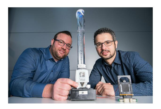
Engineers Philipp Linnebach (left) and Steffen Hau (right) from the research team led by Professor Stefan Seelecke with prototypes of a motorless pump (center) and a smart valve (front right) made from electroactive polymer film. Credit: Oliver Dietze
