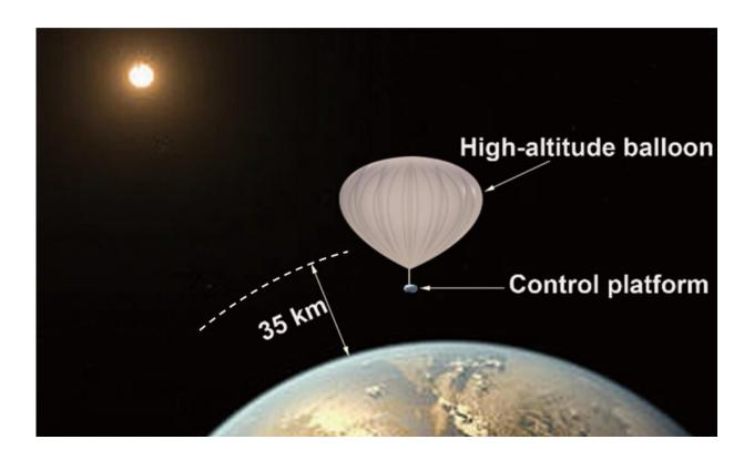
Representative schematic of the high-altitude balloon in near space (perovskite solar cells were fixed on the control platform). Credit: Science China Press
