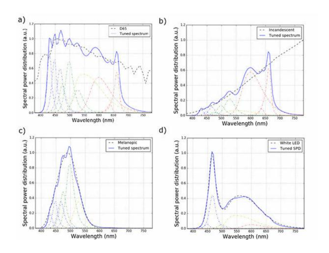
These four examples show (a) the best fit (blue solid line) to daylight D65, (b) an incandescent spectrum, (c) the melanopic, and (d) a white LED spectrum (Ph-LED YAG) (dashed black lines) made by optimizing the weights of the 10 different channels of the LED light engine (colored dash-dot lines). In all cases,
