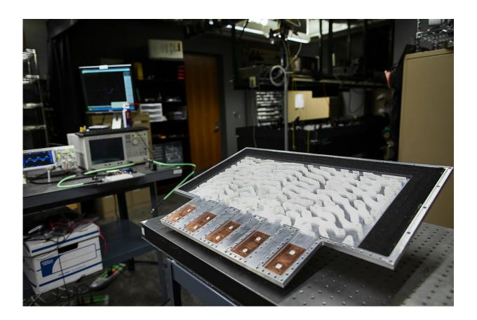
University of Pennsylvania Engineers have designed a metamaterial device that can solve integral equations. The device works by encoding parameters into the properties of an incoming electromagnetic wave; once inside, the device's unique structure manipulates the wave in such a way that it exits encoded with the solution to a pre-set integral equation for that arbitrary input. Credit: Eric Sucar
