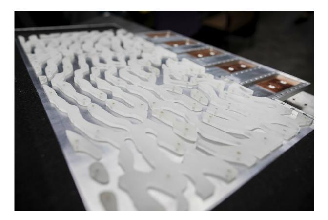
In this detail shot, the researcher's "Swiss cheese" pattern can be clearly seen. The pattern is milled out of a type of polystyrene plastic. Its complicated shape represents part of a specific integral equation that can be solved for different variables, which are encoded in the microwaves sent into the device. Credit: Eric Sucar
