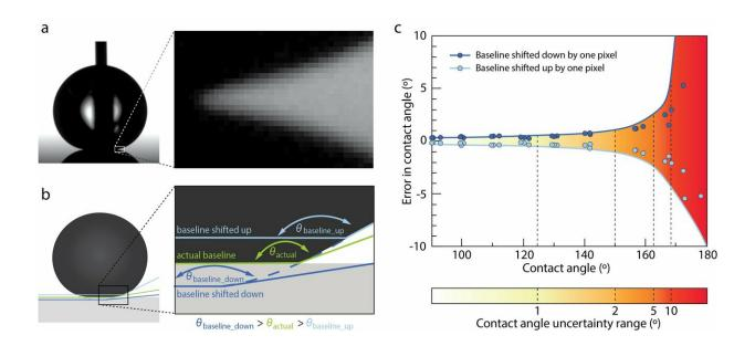
For extremely water-repellant surfaces with high contact angles, small errors in where the baselines is chosen can have substantial effects on the measured result. Credit: Maja Vuckovac
