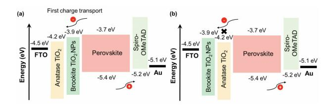
Schematic illustration the energy-level alignment between the device components with (a) FTO-AB and (b) FTO-BA as the ETLs. Credit: Kanazawa University
