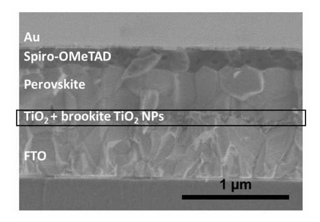
Cross-sectional SEM image of the PSC with an FTO-AB heterophase junction ETL. Credit: Kanazawa University
