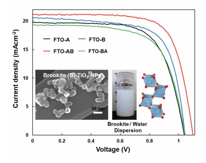
J-V curves of PSCs with FTO-A, FTO-B, FTO-AB, and FTO-BA as the ETL. Inset images: STEM image of brookite TiO2 NPs, brookite dispersion and crystallographic structure of brookite TiO2 with highlighted TiO6 polyhedral (blue and red atoms represent titanium and oxygen, respectively). Credit: Kanazawa University
