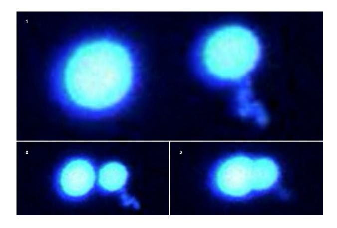
Two protein droplets refuse to merge when pushed together (fluorescence microscope images 1-3, shown sequentially). The droplets, made from fused in sarcoma proteins, are in a hard, gel-like state as they sit in a solution crowded with other molecules. Scientists used state-of-the-art optical tweezing technology to grab and manipulate these protein micro-droplets. Credit: Priya Banerjee Lab at UB
