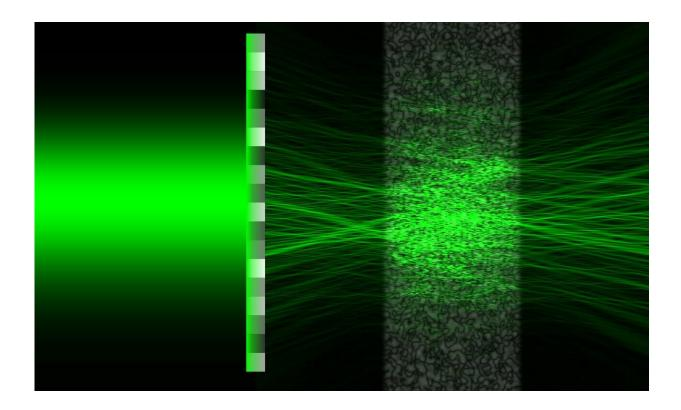
By shaping its spatial wavefront, a laser beam can propagate through a strongly scattering medium without lateral diffusion. In addition, the backscattering of light is suppressed. Credit: Yale University
