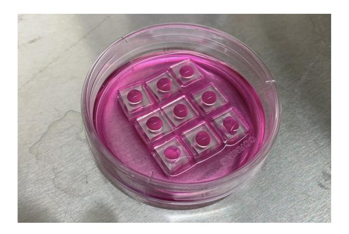
Nine nanoEP experiments in a Petri dish. The new platform can be used to infuse large proteins and pieces of DNA into cells to modify genes or label cellular activity. Credit: Yuhong Cao
