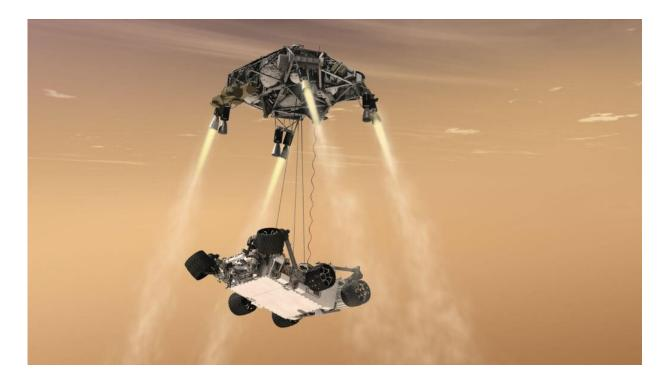
Illustration of Curiosity's skycrane, gently placing it on Mars. Credit: NASA/JPL
