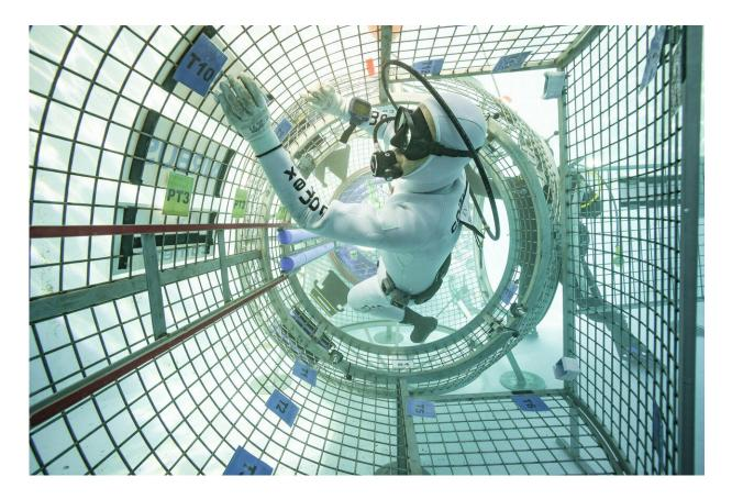
Subjects test a concept for the scientific airlock which will form part of Europe's ESPRIT module for the Gateway – a new habitable outpost near the Moon. Testing underwater enables the team to recreate the weightlessness of space. Credit: European Space Agency
