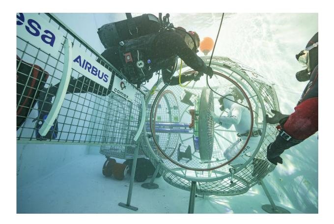
This image shows the underwater testing of one preliminary airlock design constructed by French company Comex for Airbus. The mock-up was tested underwater at Comex's facilities in Marseilles, France to simulate the weightlessness of space. Credit: European Space Agency
