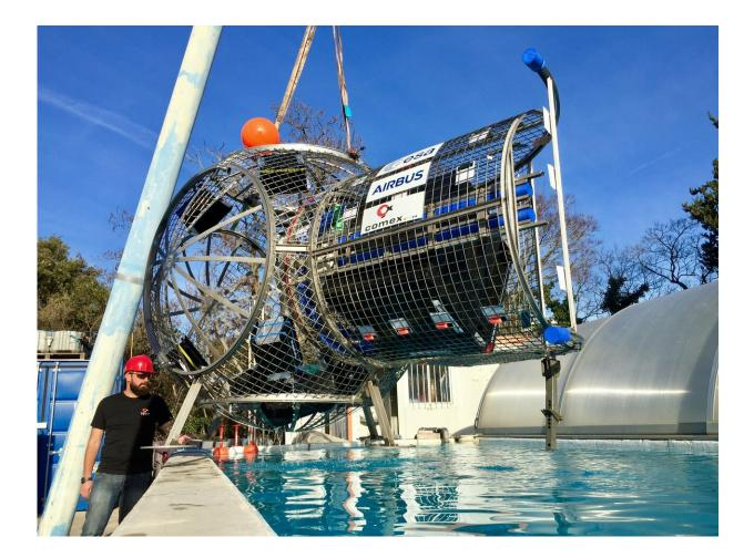
A possible design for a scientific airlock that could form part of Europe's ESPRIT module on the Gateway is lowered into a test pool by members of an
