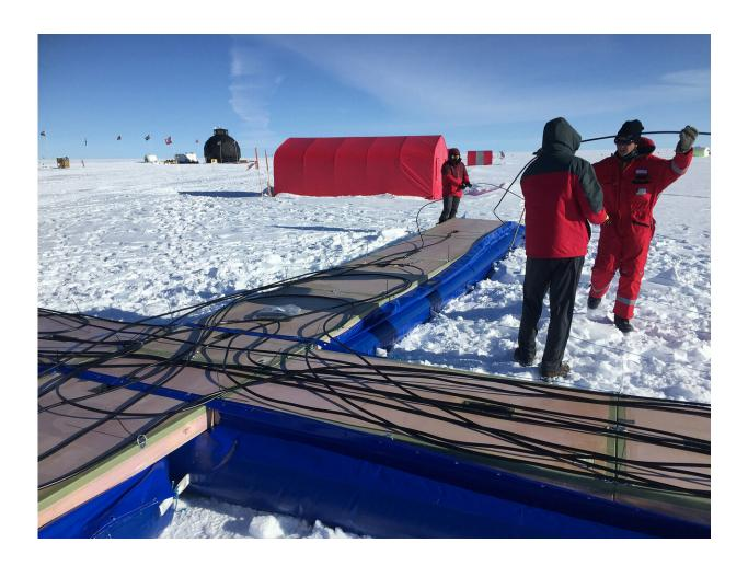
UA engineering researchers built a large antenna and a unique radar to image the bottom of an ice stream in Greenland. Credit: Dr. Stephen Yan
